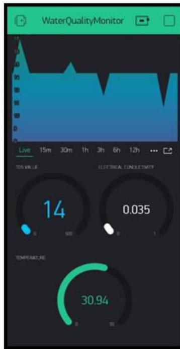
**Fig-7:** Blynk App with readings of a water with salt. The above picture shows the readings of the water with salt and graph based on the readings previously obtained.
