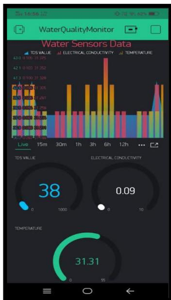
**Fig-5:** Blynk App with readings of a medicine powder. The above picture shows the readings of medicine powder and graph based on the readings obtained.
